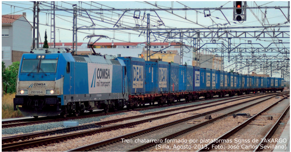
N33408 Portacontenedores Sgnss / MMC3E Takargo Rail Sgnss 38 94 455 2 012-2
