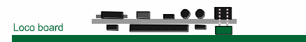
21-pin decoder plugged into loco board, i.e. TRIX Plugged in right side up, pins of the loco board penetrate through the decoder board into the socket.
