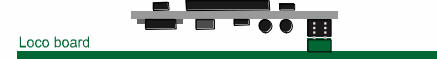
21-pin decoder plugged into loco board, i.e. BRAVA Decoder is plugged in upside down !
