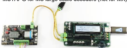
a wired decoder for SW update, sound loading, testing at MSTAPK; connection to MXULFA via "rail", software and sound projects from USB stick.
