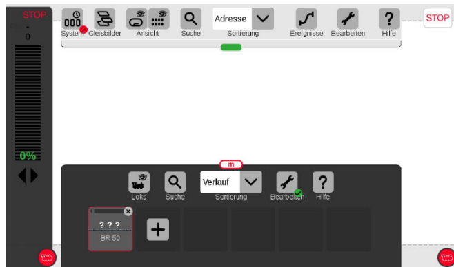
The registration was successful; loco name (in case of a sound collection: name of the first loco type, i.e. “BR 50”) is displayed. However, no picture is displayed. Instead “???”. NOTE see above!
