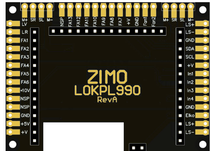
The loco board for the large scale decoder MS990L (shown in smaller scale)
